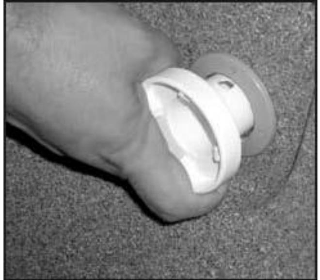
2. Insert the long part of the jet wrench and turn counter clock wise until there is no tension.
