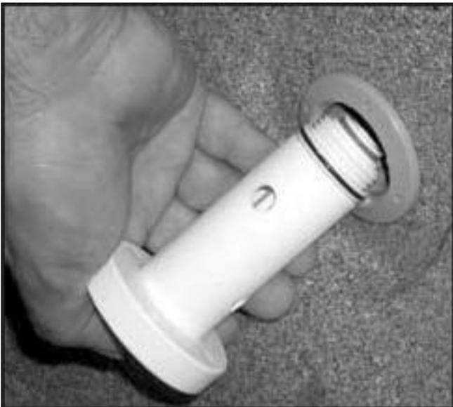
3. Remove jet wrench and jet internal nozzle assembly. Inspect condition and lubricate O-rings as needed.
