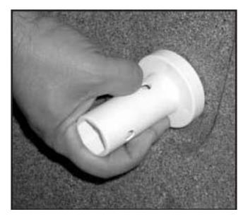
4. It is recommended to check and readjust the jet wall fitting using the short end of the jet wrench at least twice per year.
