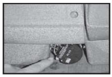
Find G.F.C.I. power plug located below the right corner of the equipment access door and cut the white tie.
