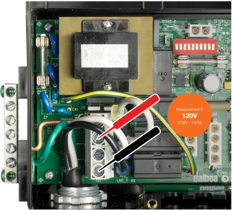
Verify the fuse (F2) is good by measuring voltage between the terminal block and the fuse. Set the volt meter to AC voltage. Measure voltage on both sides of the fuse.
