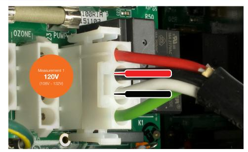
**C** - While the system is in Priming Mode, turn on the high speed pump by pressing the pump button on the topside panel. When the high speed pump is ON, measure the voltage between the red and white wires on the J23 pump connector. If the voltage measurement is 120V, the pump is bad. Replace the pump.
