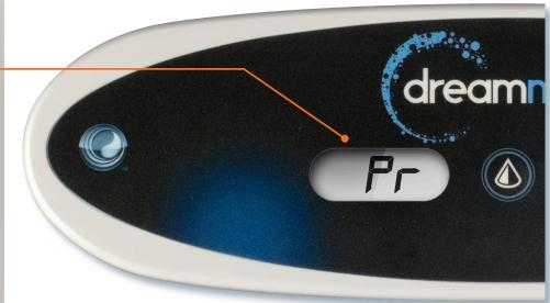
A - Once the system is powered up, it should go into Priming Mode ("Pr") automatically.
