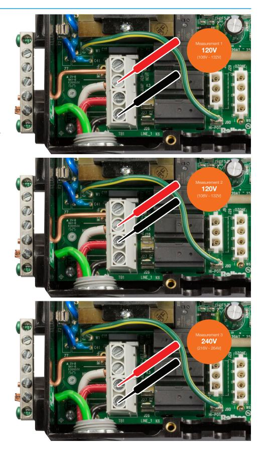
Verify the fuse (F2) is good by measuring voltage between the terminal block and the fuse. Set the volt meter to AC voltage. Measure voltage on both sides of the fuse.
