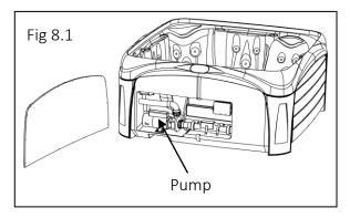
The pipes entering and leaving the pump are connected with large plastic unions. To purge the air from the pump, one of these unions will be slightly loosened.
